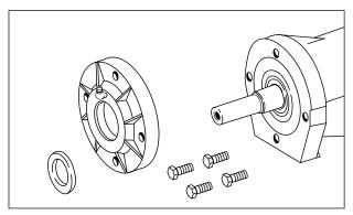
G. Bearing Cap and Slinger Removed.
